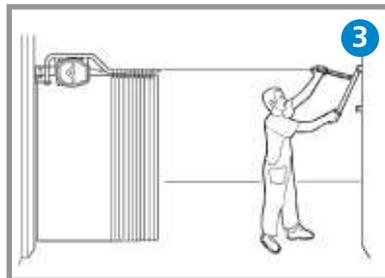
3. Hook the handgrip-ring to the tensioning lever fixed on the opposite wall of the cable reel.
